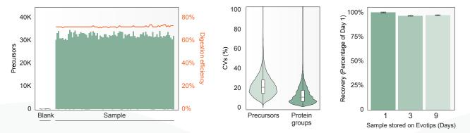
*Figure 2:* Workflow reproducibility and peptide digest sample storage on Evotips. Staring amount was 1 µg lysate and ~20% of the resulting peptides were loaded on Evotips and analyzed with 100 SPD.
